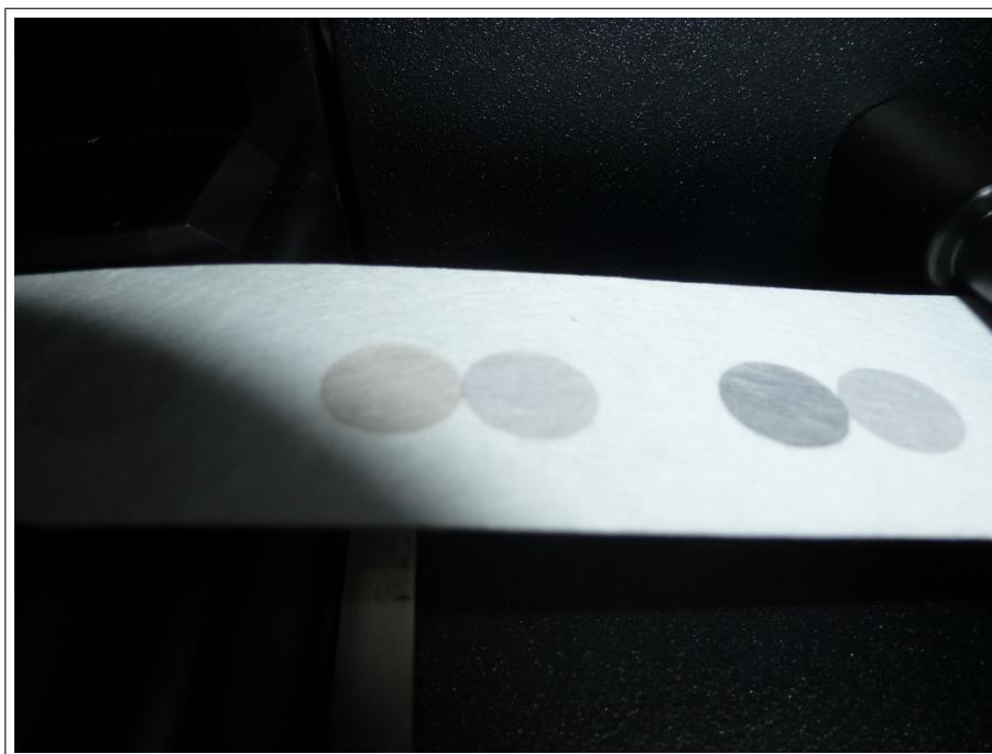
Figure 1: New spot from AE33 (S07-00729) on filter tape.
