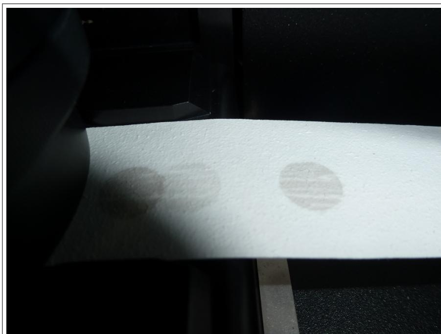
Figure 1: New spot from AE33 (S02-00204) on filter tape.
