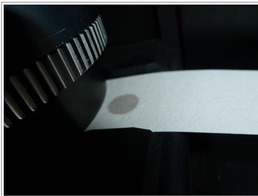
Figure 1: New spot from AE33 (S00-00055) on filter tape.
