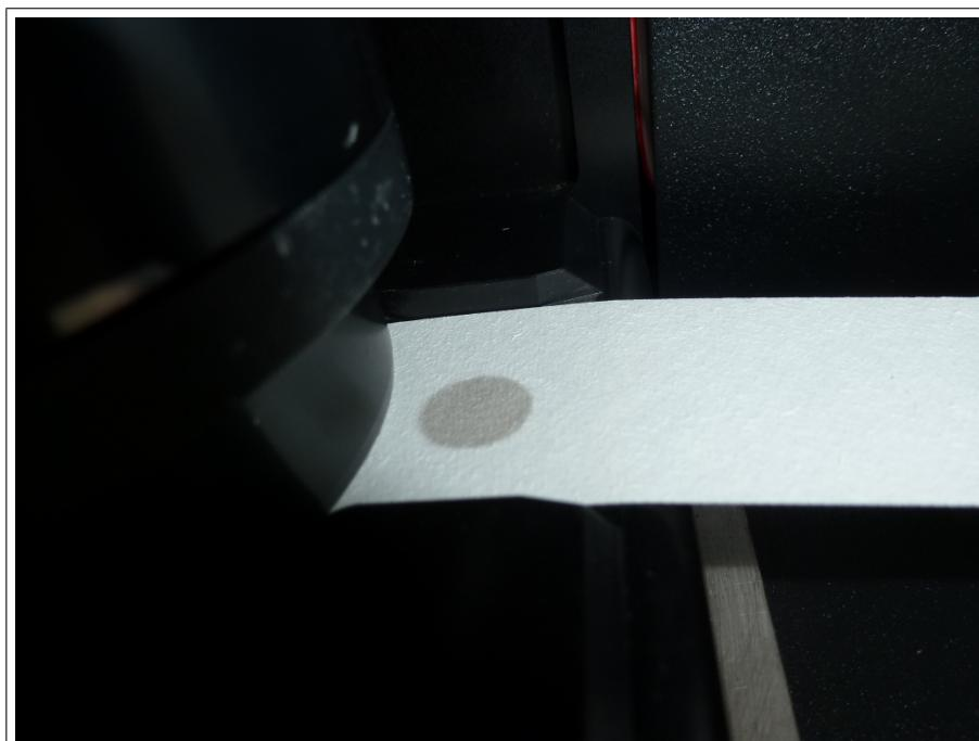
Figure 1: New spot from AE33 (S02-00156) on filter tape.
