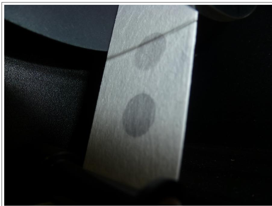
Figure 1: New spot from AE33 (S04-00387) on filter tape.
