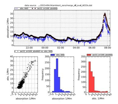
Figures: Absorption from AE33 versus multiwavelength reference absorption.
