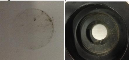
**Recommendations:** External sensor cable should be replaced. The whole inlet system of the measurement station should be check for dirt inside aerosol lines.
