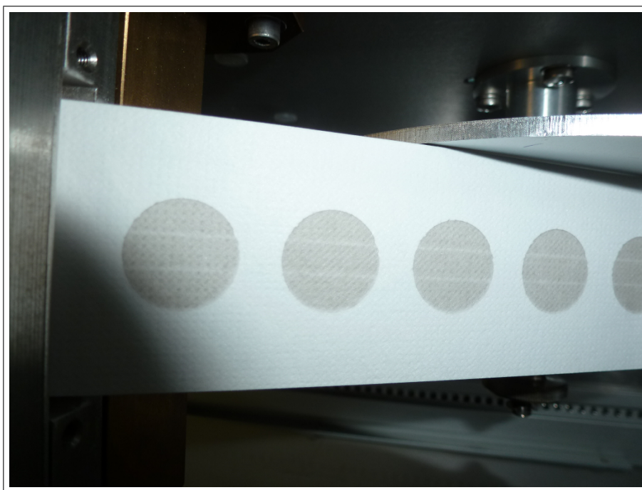
Figure 1: New spot from MAAP (42545) on filter tape.
