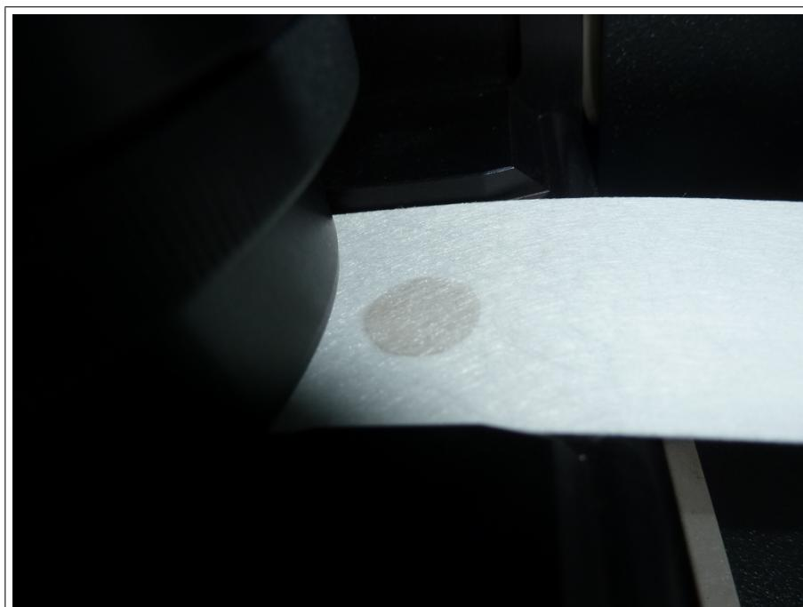
Figure 1: New spot from AE33 (S07-00636) on filter tape.
