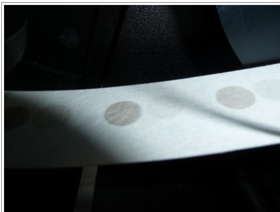
Figure 1: New spot from AE33 (S02-00202) on filter tape.
