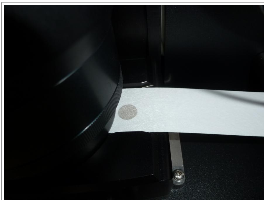
Figure 1: New spot from AE33 (S07-00705) on filter tape.
