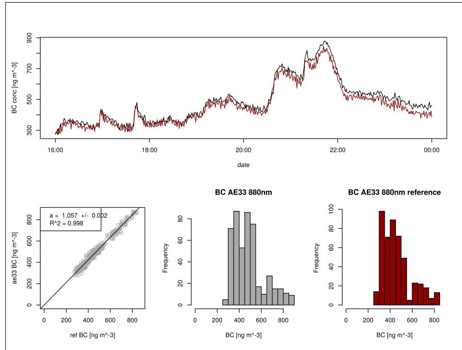
Figure 3: Correlation of eBC coefficient (BC6) from AE33 (S07-00705) and reference AE33.
