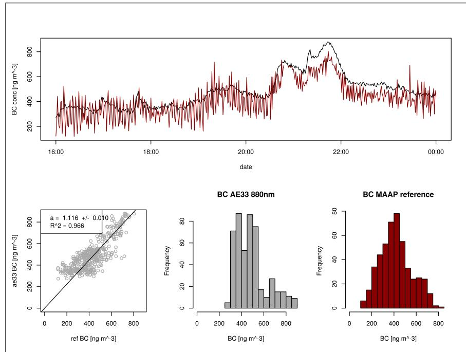
Figure 2: Correlation of eBC coefficient (BC6) from AE33 (S07-00705) and reference MAAP.
