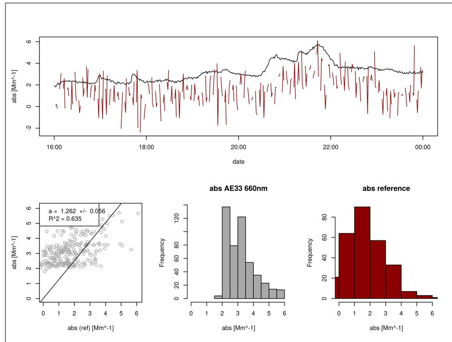
Figure 4: Correlation of absorption from AE33 (S07-00705) and the multi-wavelength absorption reference at 660 nm.
