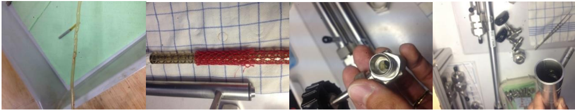
Figure 01: Status of the nafion membrane. The nafion membrane is completely damaged from the sea salt and it is also broken in two pieces.
