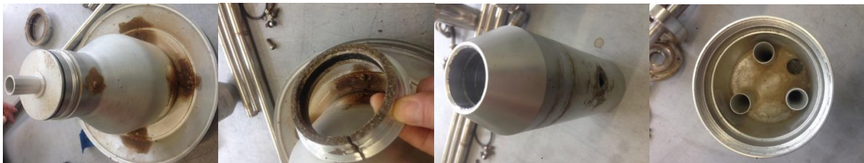
Figure 02: Status of the PM10 head. There was heavy corrosion on the supporting screws and ring. Screws and aluminium net were replaced.
