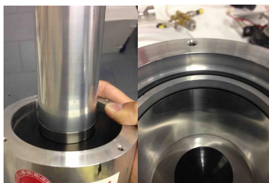
Figure 04: DMA status: The DMA was opened and completely cleaned.
