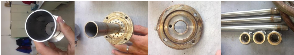
Figure 03: Splitter and SS piping. The splitter was sand blasted and the piping and fitting were replaced.
