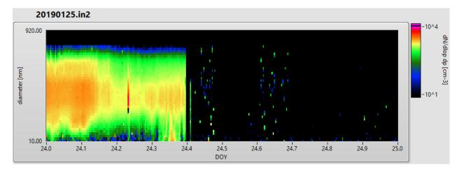
Fig 5: Lack of CPC working fluid
