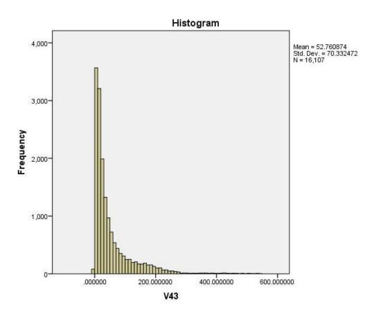
Fig. 8: But the histogram reveals almost 100 values less than zero due to inversion artefacts
