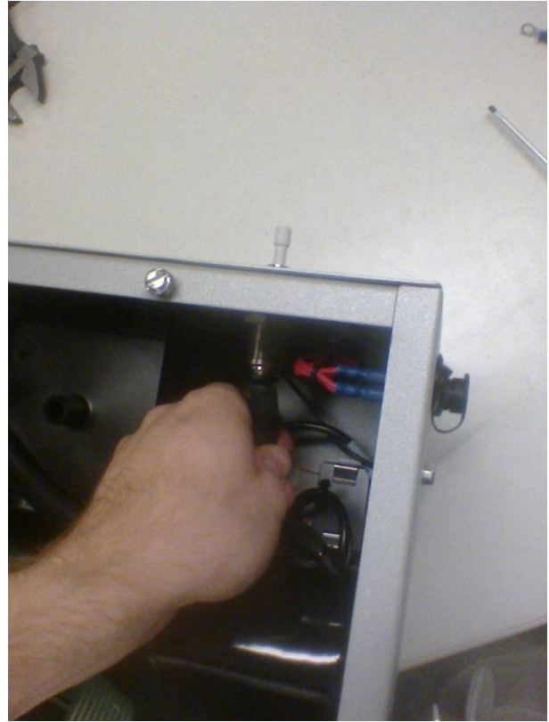
Figure 13. Removing the exhaust hose from the blower and connecting it to the external pump connector.
