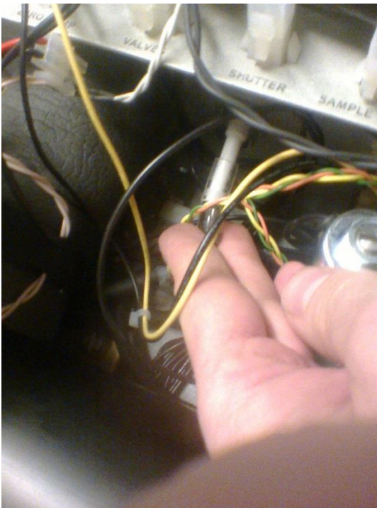
Figure 3. Plugging the zero air hose.
