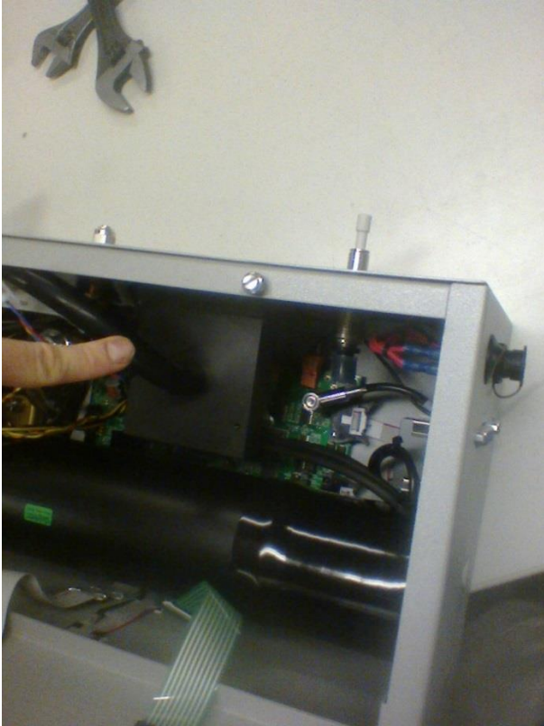
Figure 13. Removing the exhaust hose from the blower and connecting it to the external pump connector.
